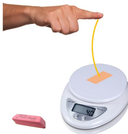
Figure 1: The force that causes the onset of buckling is determined from the mass reading on the digital scale.
